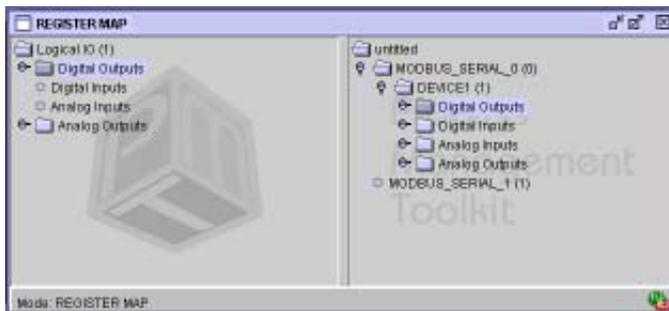
The Logical Memory Map is used to map all physical I/O to the correct register range in the RDP180's Logical Memory Map.
