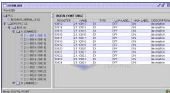
I/O Builder is used to configure communication parameters for the RDP180's serial ports. Use this module to add and configure the devices that the RDP180 will interface with, including Modbus master and slave devices.
